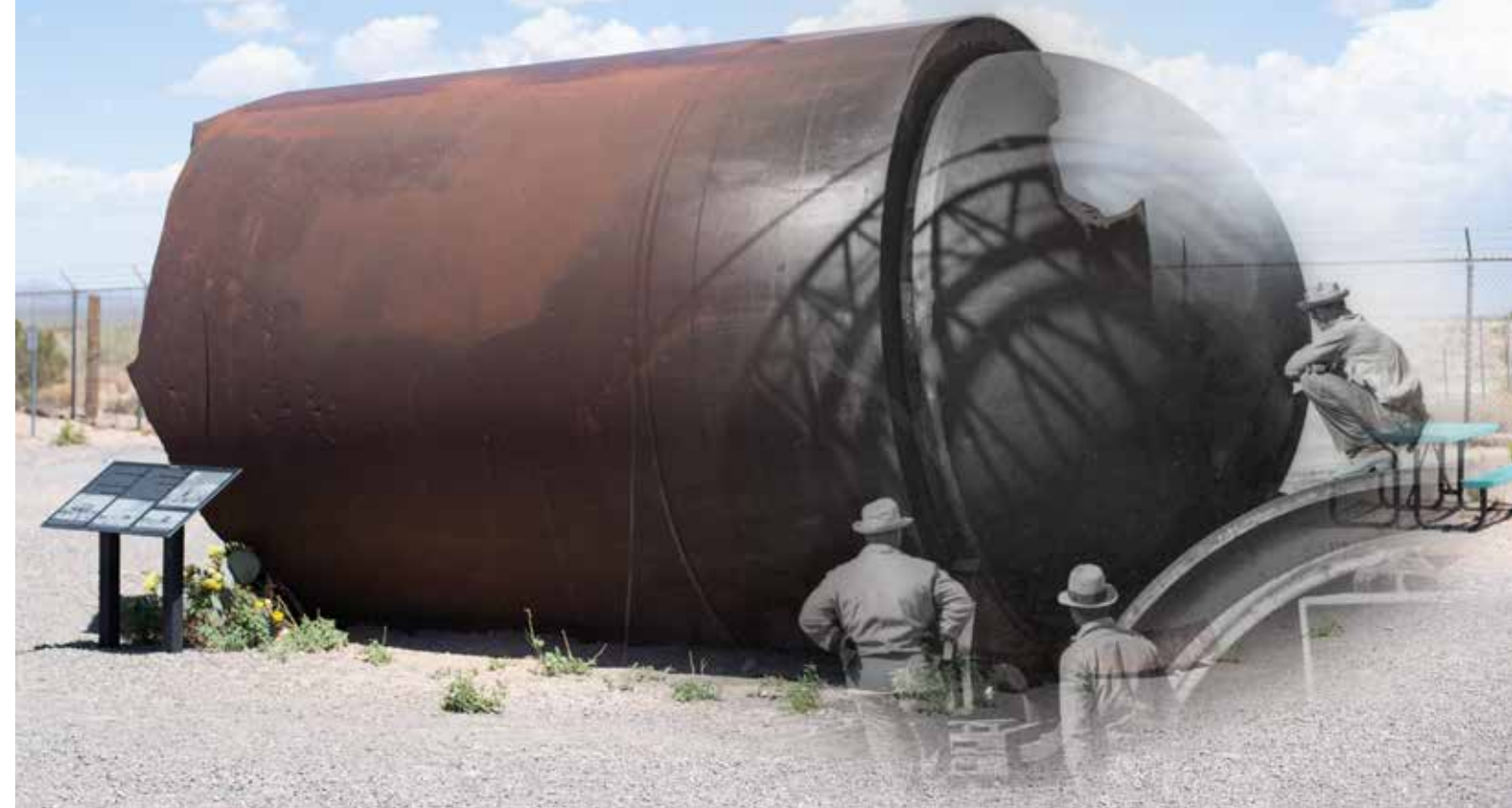
▲ Manufactured in Ohio by Babcock & Wilcox, Jumbo was originally 25 feet long, 10 feet in diameter, and weighed 214 tons. Scientists planned to use Jumbo to contain the Trinity test but then changed their minds. (For more, see “About the cover” on p. 1.)
